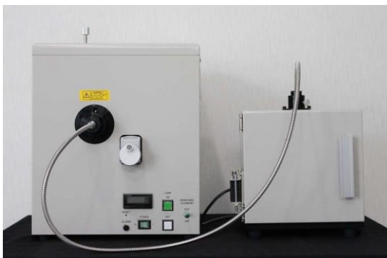
EQE (IPCE) measurement setup (desk top size)
