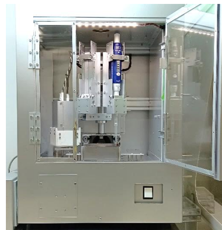
Automatic spin coating robot (wireless control, atmosphere changeable)
